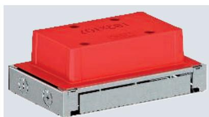
Underfloor outlet box with fixed, unchangeable 106 x 182 mm installation opening for an installation unit of nominal size 2. The mounting opening is created using the screed protection cover contained in the scope of supply. The underfloor box has two openings for M20 conduit on the narrow sides. The underfloor box is suitable for screed floor constructions with height 70 mm up to 90 mm.
