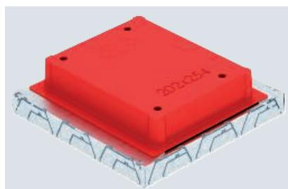
Underfloor outlet box with fixed, unchangeable 202 x 254 mm installation opening for an installation unit of nominal size 6. The mounting opening is created using the screed protection cover contained in the scope of supply. The underfloor box possesses installation openings for three single-compartment PVC ducts of nominal size 60 x 25 and 90 x 35 on all four sides. The box is principally suited for use in floor structures in cement screed with a structure height of up to 90 mm.
