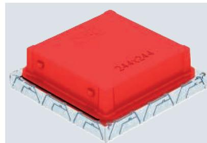
Underfloor outlet box with fixed, unchangeable 244 x 244 mm installation opening for an installation unit of nominal size 9. The mounting opening is created using the screed protection cover contained in the scope of supply. The underfloor box possesses installation openings for three single-compartment PVC ducts of nominal size 60 x 25 and 90 x 35 on all four sides. The box is principally suited for use in floor structures in cement screed with a structure height of up to 100 mm.
