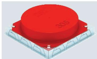
Underfloor outlet box with fixed, unchangeable installation opening of Ø 305 mm for an installation unit of nominal size R9. The mounting opening is created using the screed protection cover contained in the scope of supply. The underfloor box possesses installation openings for three single-compartment PVC ducts of nominal size 60 x 25 and 90 x 35 on all four sides. The box is principally suited for use in floor structures in cement screed with a structure height of up to 95 mm.
