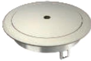
Service outlet with blanking cover and Allen screw with locking slider for GES R2 floor socket for direct installation in the MT R2 installation socket. The cover version can be used as a cable outlet. When closed, the floor socket fulfils the requirements of EN 50085-2-2 for wet-cleaned floors.
