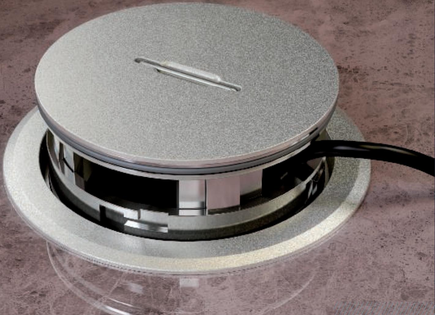
The tube body seals the closed installation space against the ingress of water, which occurs, for example, when the floor is cleaned. Even if the tube body cover is open for letting out cables, a seal in the lower ring of the installation socket offers protection against the ingress of water. The GES R2 floor socket with tube body thus fulfils the requirements for service outlets in wet-care floors according to EN 50085-2-2 and is certified to IP66 in the unused state.
