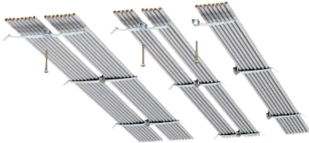
The tested pressure clips are suitable for installation in the false ceiling area of escape and rescue routes. In the event of fire, the pressure clips have a proven mechanical stability of 30 minutes. They are mounted under the ceiling. The pressure clips are made of sprung, rustproof
