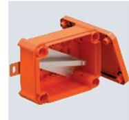
Unequipped, closed connection or junction box for free termination with ceramic terminals and cable glands. Dimension A indicates the available support rail length for the wiring terminals. Sufficiently large wiring compartment through diagonally arranged support rail. Fastening on easily accessible external flaps made of stainless steel. Approved for cable systems that maintain the electrical function according to DIN 4102 Part 12 with the classes E30, E60 and E90.
