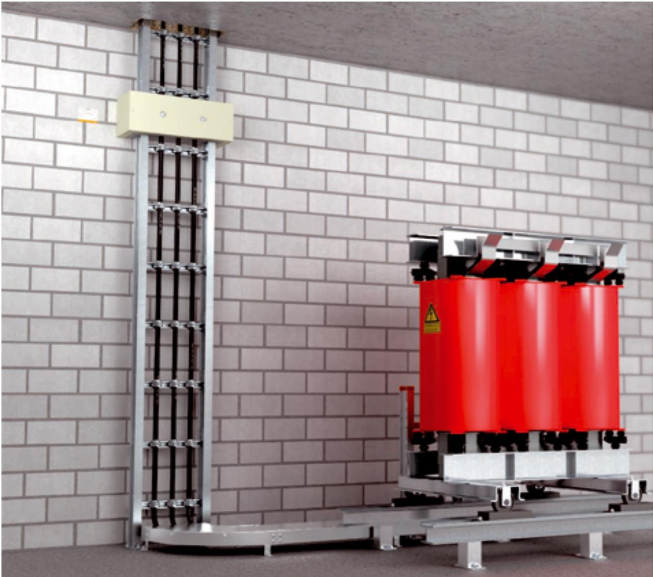
OBO vertical ladder systems for vertical routing of all kinds of cables. Available as light-duty vertical ladders with a side height of 45 mm, as a heavy-duty vertical ladder with U profiles and as industrial vertical ladders with I profiles. Both the heavy-duty and industrial vertical ladders can be assembled in variable lengths. The side rails are standard profiles of type US 5 and IS 8, which are
