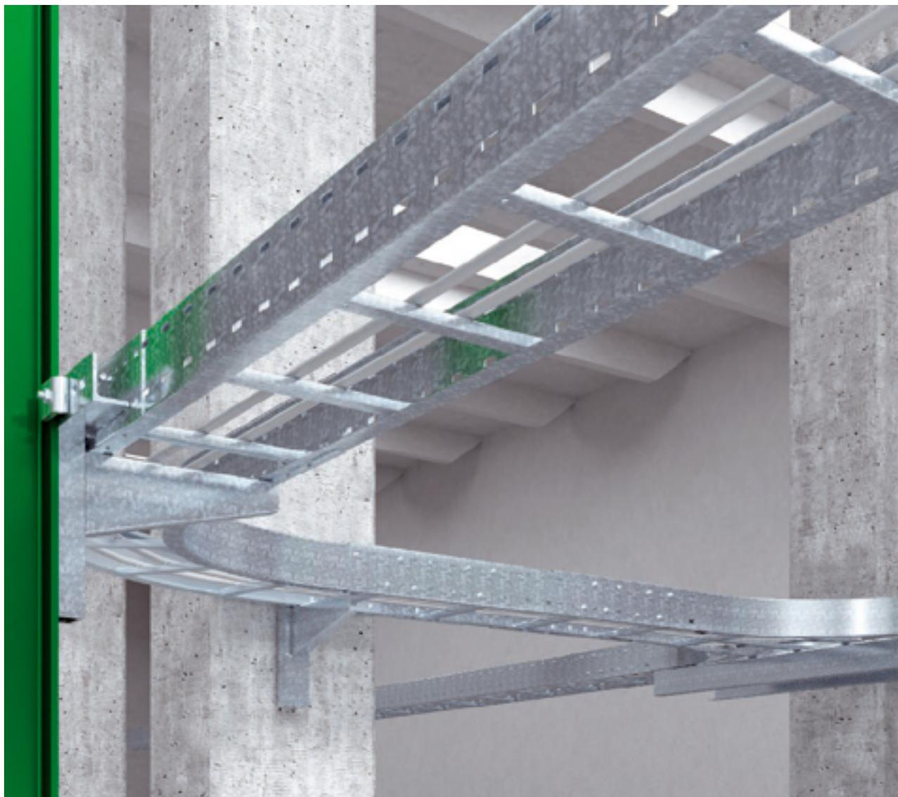
When you need to bridge wide spans and support high cable loads, the OBO wide span cable ladders are the perfect solution. The product range comprises wide span cable ladders with widths of between 200 and 600 mm and side heights of 110 to 160 mm. Comprehensive system accessories, such as fittings and all the fastening materials for concrete and steel mounting, round off this product range perfectly. OBO wide span cable ladders
