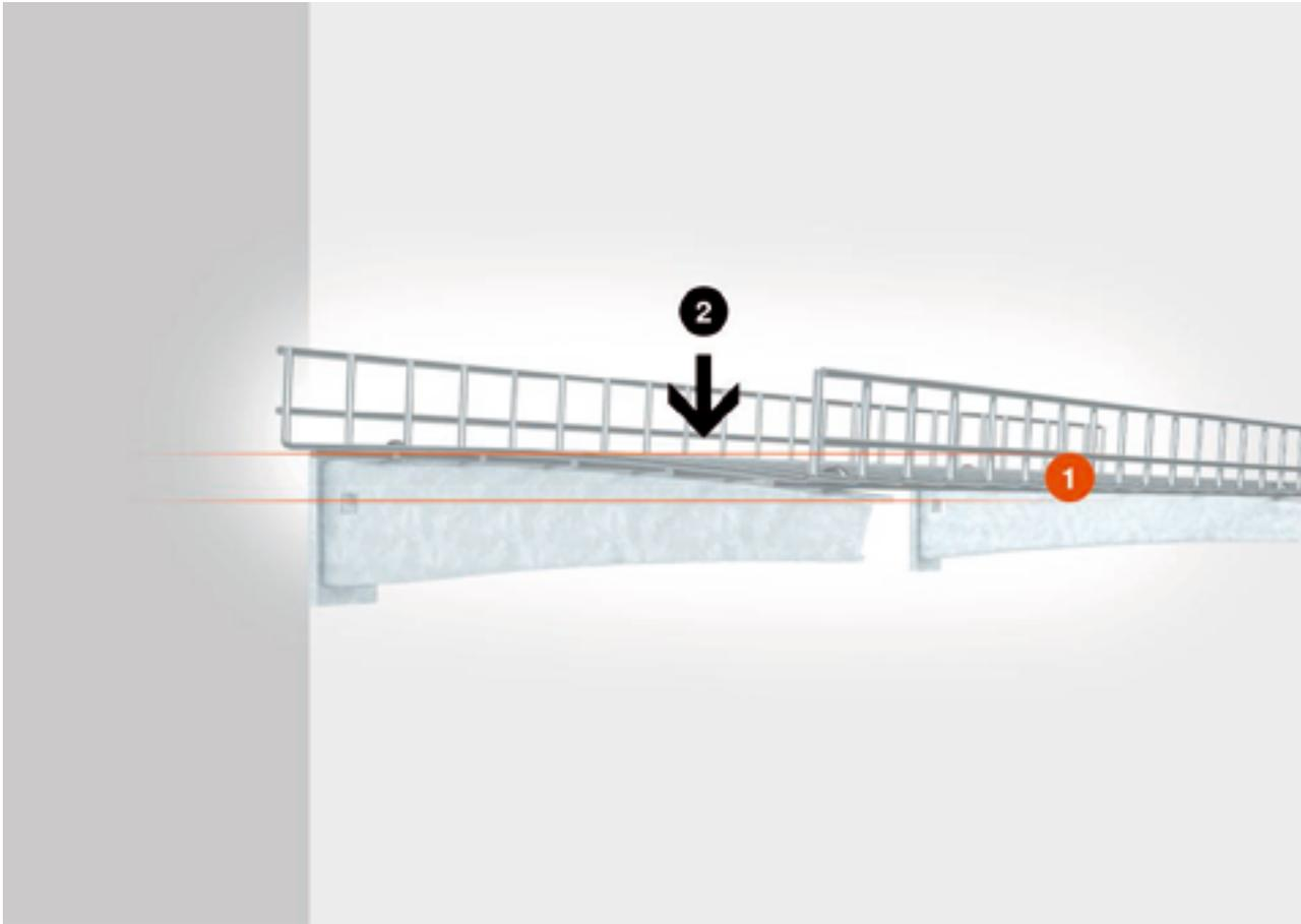
Key components of the OBO cable support systems are the parts for mounting, in particular the brackets and suspended supports. They connect the cable trays and ladders to the wall and to the ceiling, and are thus an important construction element of the overall system. When calculating the load capacity of a cable support system, the brackets and suspended supports must not be forgotten. The test diagram is also useful in selecting the right products.
