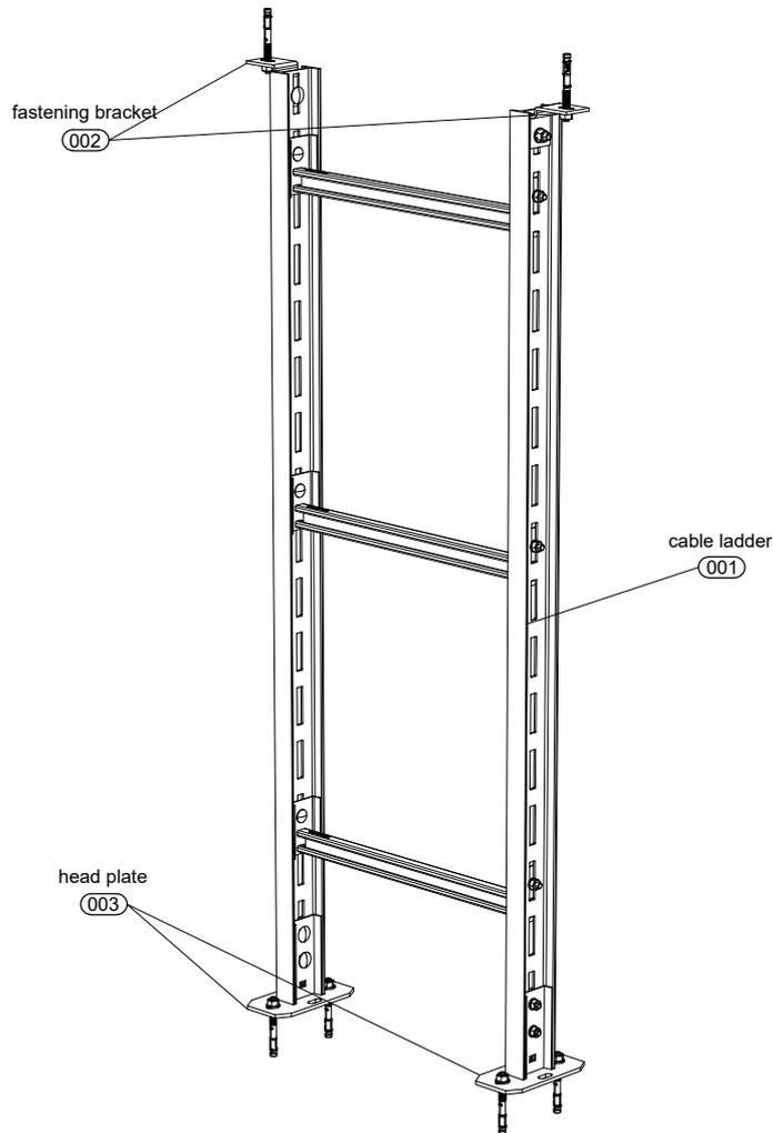
This free-standing cable ladder is suitable for single-sided cable clamp installation.
