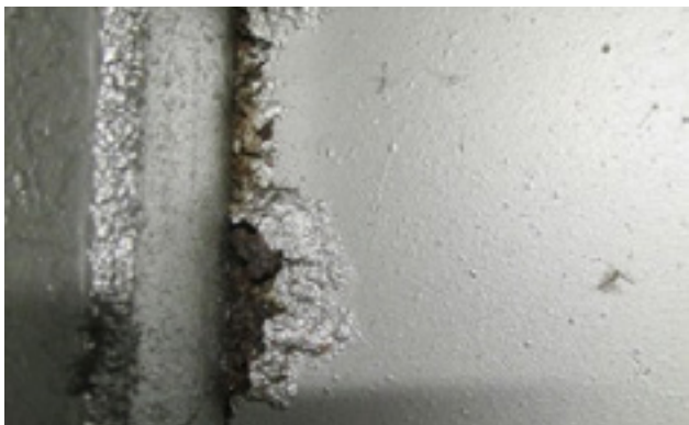
Gap corrosion on an enclosure. Through the progressing underlying rust the coating is damaged (source: OBO Bettermann)
