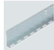
Barrier strip for the BKRS walkable cable tray system. Fastening with truss-head bolts M 6 x 12 in the base perforation.
