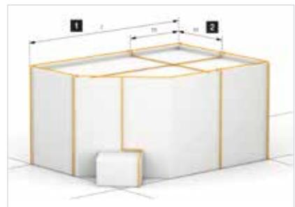
The grid method is suitable for buildings with simple shapes, e.g. with flat roofs.
