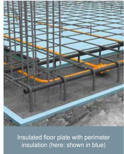
Insulated floor plate with perimeter insulation (here: shown in blue)
