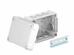
Junction box for the connection of cables and lines indoors and in protected outdoor areas. Rectangular design with plug-in seals to the sides and knock-out entries in the bottom. Suitable for wall and ceiling mounting and on mounting panels. With the option to fasten inside and to mount via the corner domes. High, transparent cover with quick lock, sealable. Made from halogen-free and UV-resistant materials.
