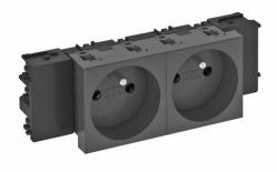
Earthing pin socket with connection to side, Double  $0^\circ$ , with increased touch protection, with screwless terminals, 2-pin, 16 A, 250 V~, with connection terminals to IEC 60884-1, suitable for the installation in Rapid 45 device installation trunking systems.
