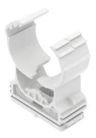
Highly stressable clip for accepting plastic or metal electrical and sanitary pipes as well as the electrical installation pipe Quick pipe. Universal fastening options on walls, ceilings and steel constructions, both indoors and outdoors. Flexible clamping range of several millimetres. Tooless pipe mounting. Connectable to
