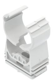
Highly stressable clip for accepting plastic or metal electrical and sanitary pipes as well as the electrical installation pipe Quick pipe. Universal fastening options on walls, ceilings and steel constructions, both indoors and outdoors. Flexible clamping range of several millimetres. Tooless pipe mounting. Connectable to
