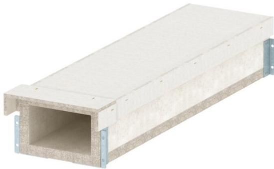
Fire protection duct made of water and frost-resistant fibreglass lightweight concrete of material class A1 according to EN 13501-1 for fireproof routing of cables in escape and rescue routes. EI30 - EI60 classification as installation duct according to EN 13501-2 on the basis of tests in accordance with EN 1366-5. When there is an internal fire load (cable fire), the duct prevents the spread of fire from one fire section to another.
