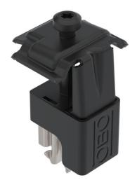
Universal clamp for mounting photovoltaic modules on flat and pitched roofs, suitable as a clamp between 2 modules or as an end clamp. Lockable pre-fastening on TP 45 support profile and on STK and STL supports. Suitable for 10 mm slot width. Can be rotated through 90° after engaging. Screwable fastening of the PV module with Torx 30 key.
