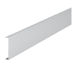
Aluminium cover, for closing Rapid GA device installation trunking and ISS service poles with a 76.5 mm system opening. The firm position of the cover and electrical contact to the lower part of the trunking and service pole is guaranteed thanks to type RKV3V locking brackets. There are 6 pre-mounted locking brackets included per delivery length (2,000 mm).
