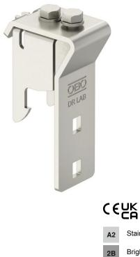
Spacer for stand-off mounting of covers on wide span cable trays and wide span cable ladders. Space height 35 mm, stainless steel 1.4301.
